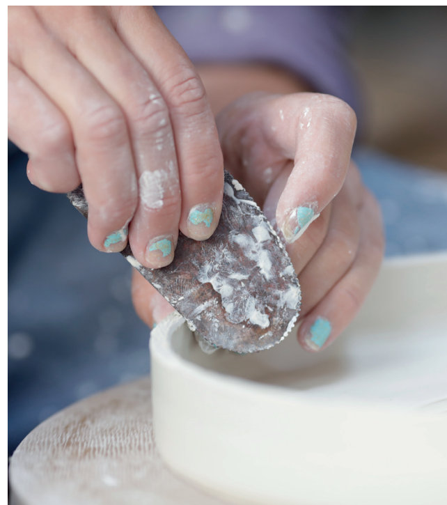
14 I have 18mm birch ply batts that fit back on the wheel with bolts on the wheel head. Using a serrated kidney, I score and cross-hatch the top edge. I then cut an angle off the inside edge to accommodate the excess slurry that will be used to join the pieces together.
