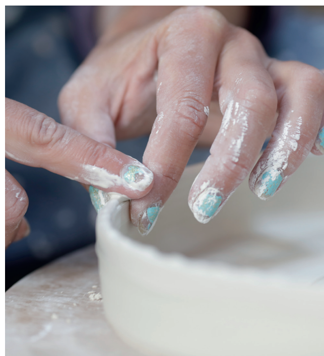
15 I agitate the slurry onto the top edge. Making a gauge with my forefinger and thumb and using the finger of my other hand on top, I apply an equal amount all the way around. This is done on both pieces.
