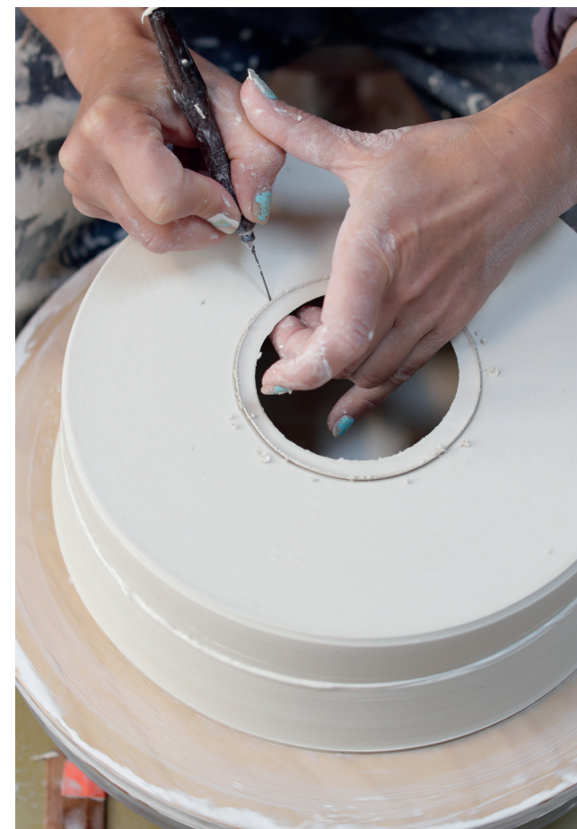
17 Slowly turning the wheel, I carefully incise the top with a pin to enlarge the hole so that it is big enough for my hand to go through.
